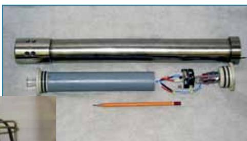
Autonomous wave and water level meter AWM (above)
