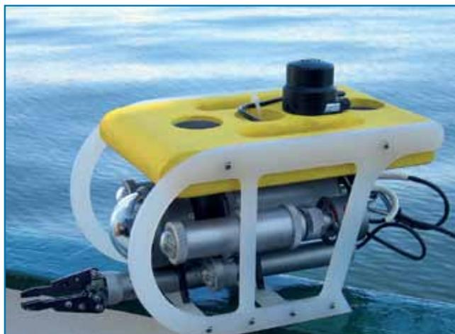
**Remote operated vehicle from the GNOM series equipped with a propulsion and steering system, a video camera, a «capture» - type manipulator and an all-round sonar**
