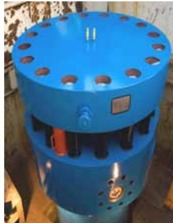
Coastal hyperbaric complex (left) and the test chamber for imitation of ocean depths up to 9 km (right) in the Southern Branch of IO RAS
